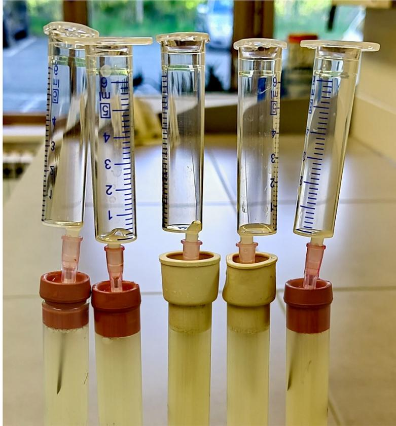
**Figure 1.1.** Experimental setup: Inserting a medical needle into a glass tube by puncturing the rubber stopper and then attaching the syringe.
